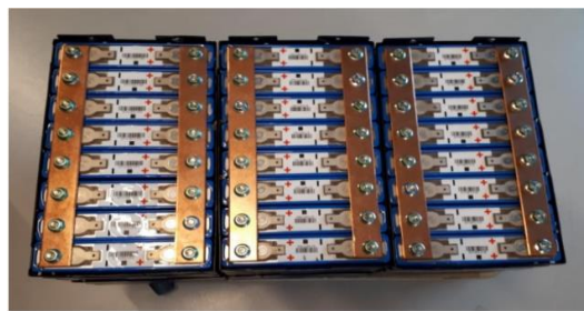
Figure 3. Internal view of 3 battery banks with 8 cells each during a test setup (parallel connection)
