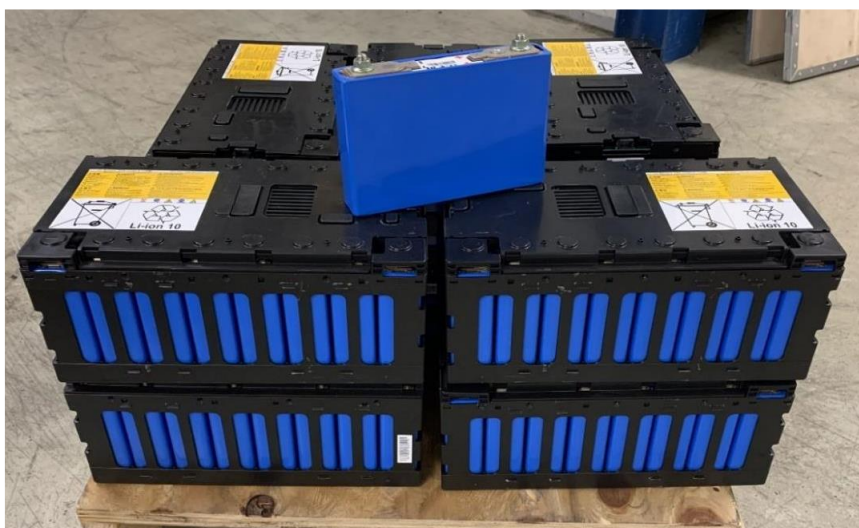
Figure 9. Battery banks with cells in series
