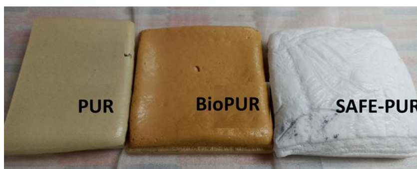
Figure 6. Demo sandwich panels made from bioPUR (left). Different varieties of PUR materials from INDRES (right).
