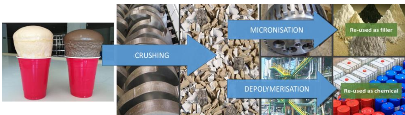
Figure 5. Mechanical and chemical recycling methods for Polyurethanes
