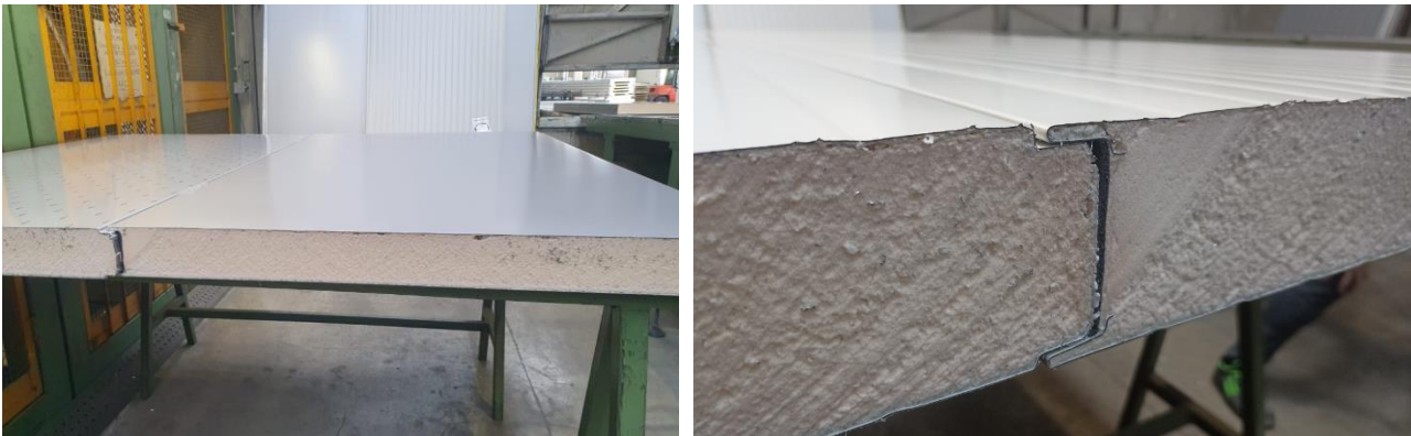
Figure 7. Roof sandwich panel manufacturing
