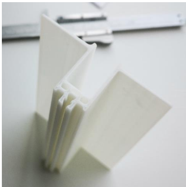
Figure 5. Upright Profile for panel-to-panel connection.
