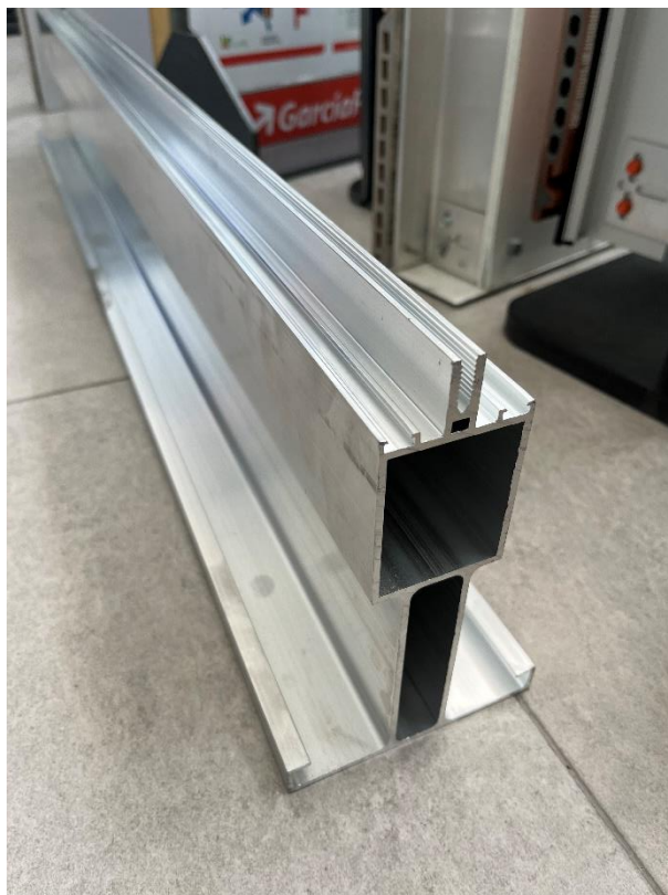
Figure 28. Image showing the test extrusion of the roof aluminium profile.
