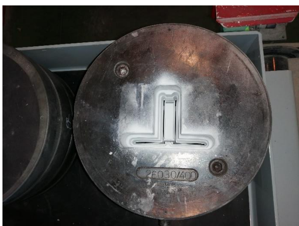
Figure 11. Extrusion dies for profile manufacturing as developed by EXLABESA for the RE-SKIN façade system.
