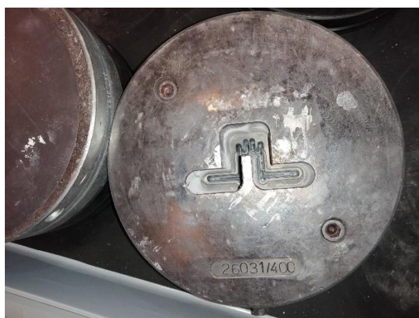
Figure 11. Extrusion dies for profile manufacturing as developed by EXLABESA for the RE-SKIN façade system.
