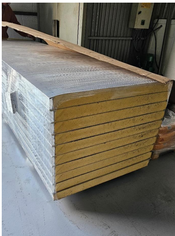
Figure 30. RE-SKIN sandwich panels manufactured for the roof
