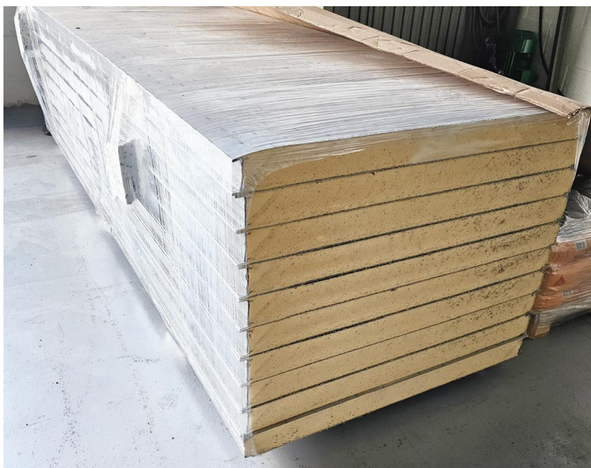
Figure 44. RE-SKIN sandwich panels manufactured for the roof
