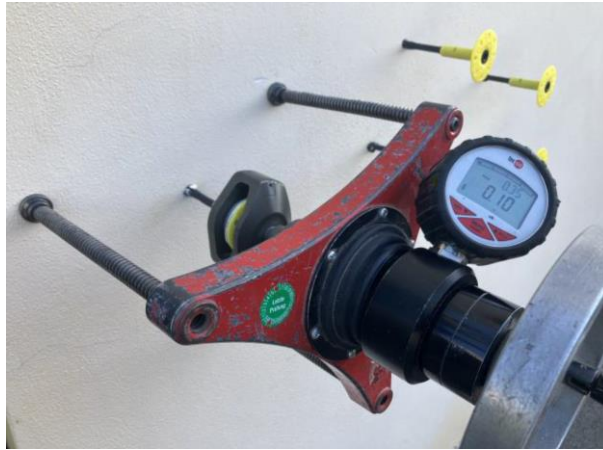
Figure 1. Dynamometric test being performed in the Milan demonstration building
