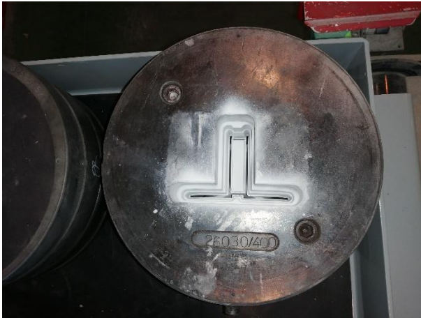
Figure 17. Extrusion dies for profile manufacturing as developed by EXLABESA for the RE-SKIN façade system.
