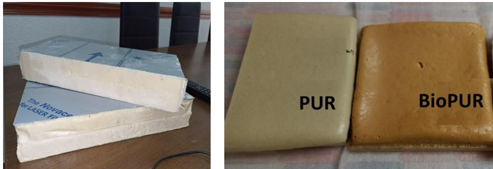
Figure 8. Demo sandwich panels made from bioPUR (left). Different varieties of PUR materials from INDRES (right).
