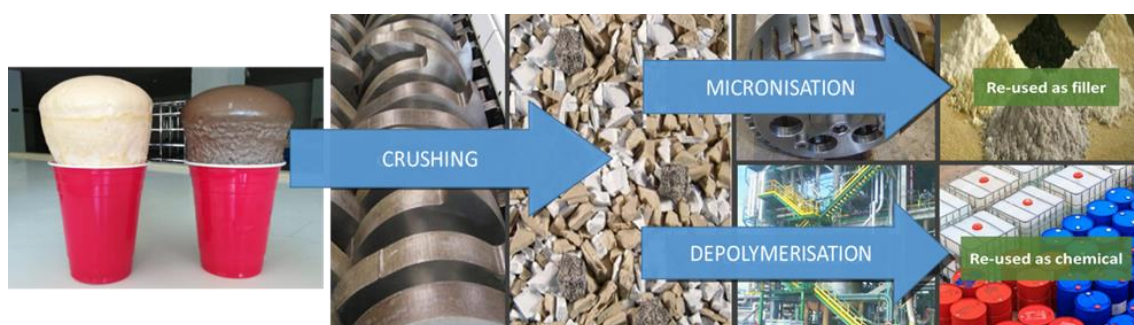
Figure 7. Mechanical and chemical recycling methods for Polyurethanes (Source: INDRESMAT)
