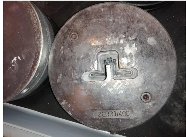
Figure 17. Extrusion dies for profile manufacturing as developed by EXLABESA for the RE-SKIN façade system.
