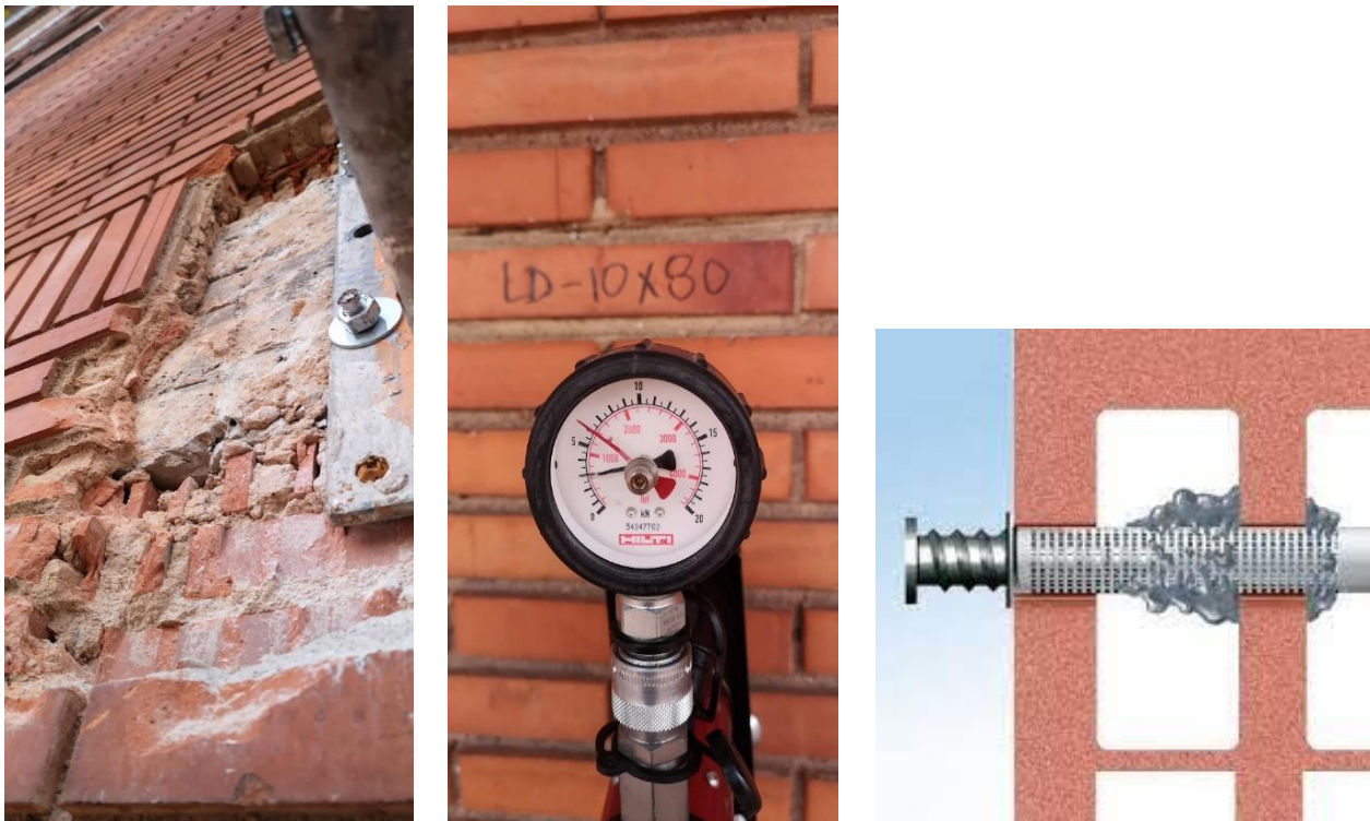
Figure 41. Dynamometric test (Pull-Off Test Guide in Annex)
