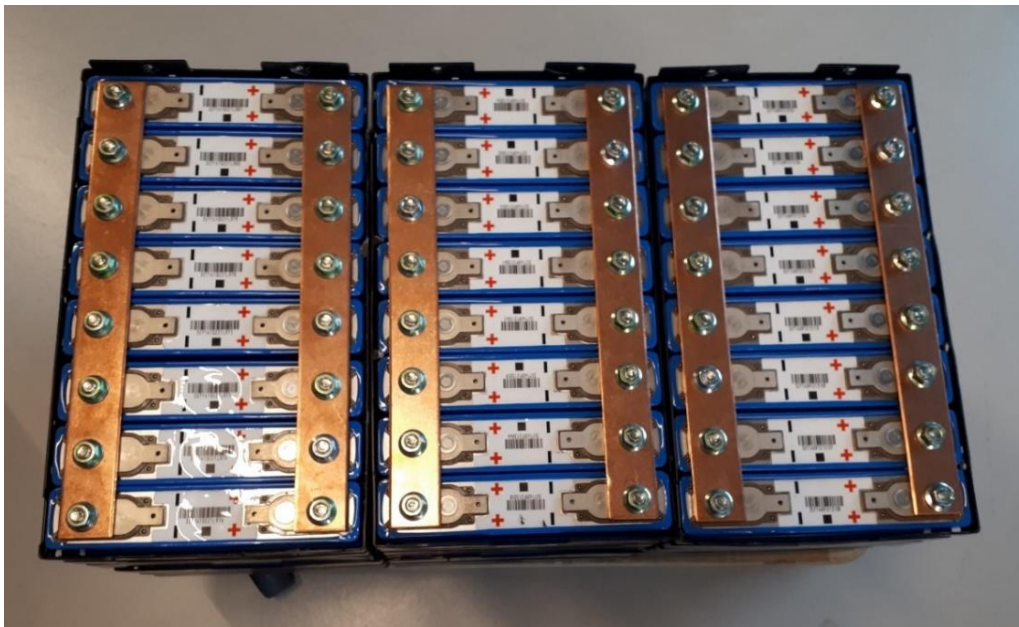
Figure 26. Internal view of 3 battery banks with 8 cells each during a test setup (parallel connection)
