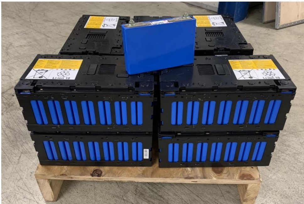
Figure 27. View of sealed battery banks with 8 cells in series with on top a single battery cell
