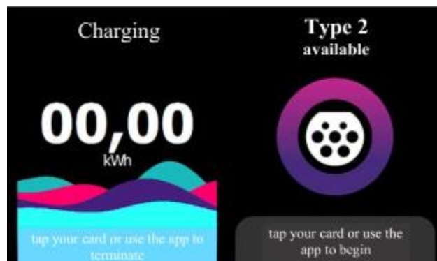
Figure 32. Display when the charging in the R side socket ends and the socket is available again
