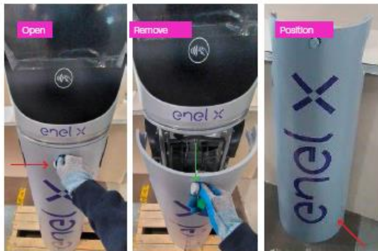
Figure 22. Version B front panel pre-dispositioning
