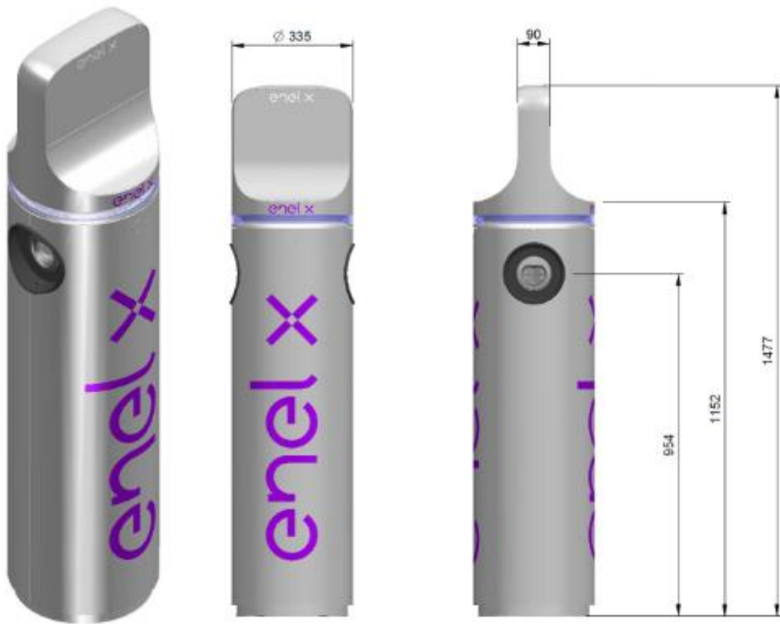
Figure 21. Version B main dimensions [mm]
