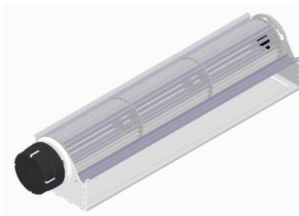
Figure 12. Fan in the fan-coil unit 3D model
