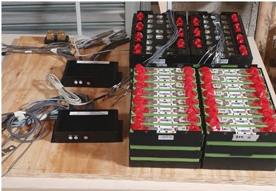
Figure 32. The components that will be installed on each shelf (2 battery slabs and 2 BMS)
