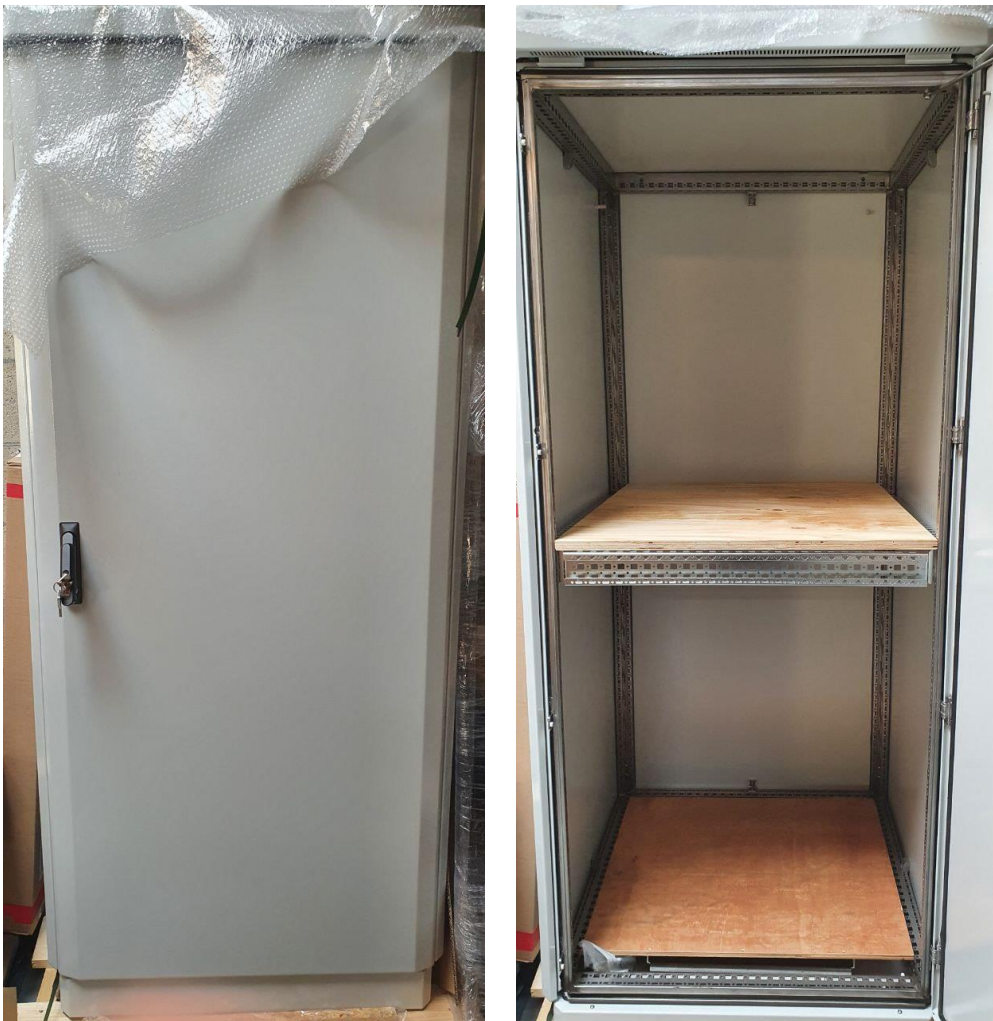
Figure 31. The updated battery enclosure, the wooden panels are placed temporarily for dimensioning and they will be replaced with metallic panels.
