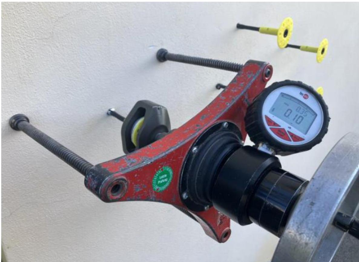
*Figura 17 – Pull-out test*
