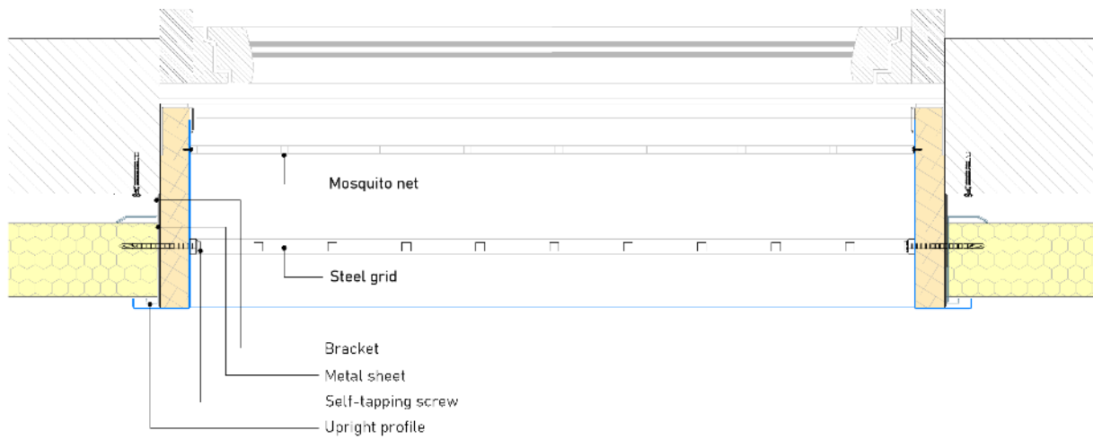
Figure 35. Detail drawing (horizontal) of the mosquito nets and steel grids in the Milan case study [drawing created using AutoCAD]
