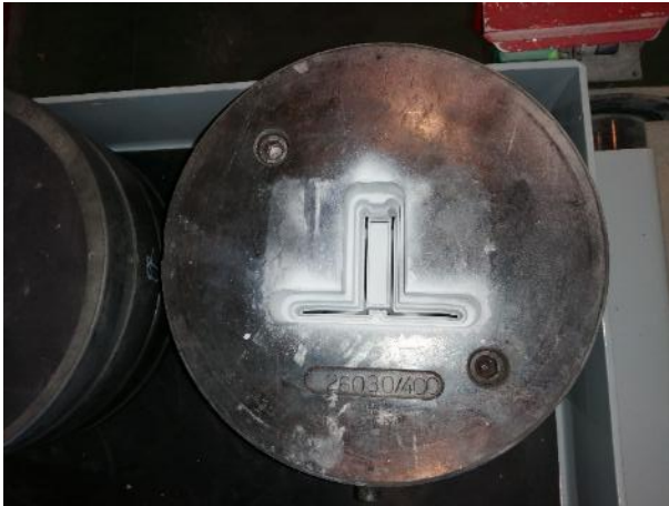
Figure 19. Extrusion dies for profile manufacturing as developed by EXLABESA for the RE-SKIN façade system.
