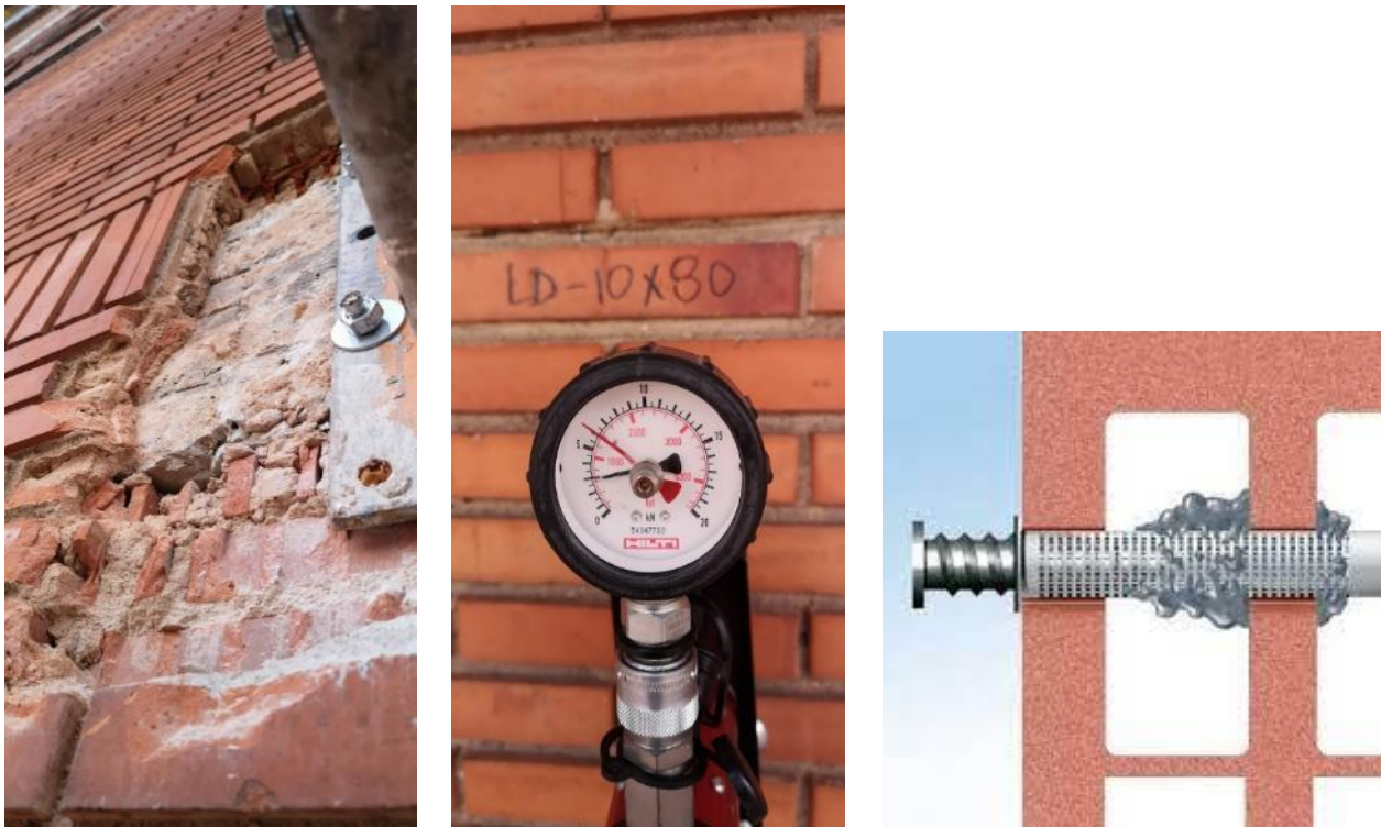
Figure 44. Dynamometric test (Pull-Off Test Guide in Annex)
