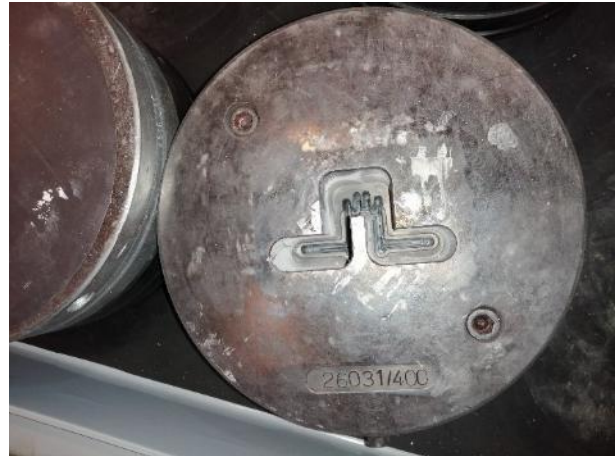
Figure 19. Extrusion dies for profile manufacturing as developed by EXLABESA for the RE-SKIN façade system.
