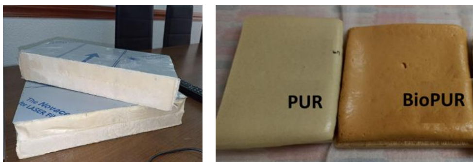
Figure 10. Demo sandwich panels made from bioPUR (left). Different varieties of PUR materials from INDRES (right).
